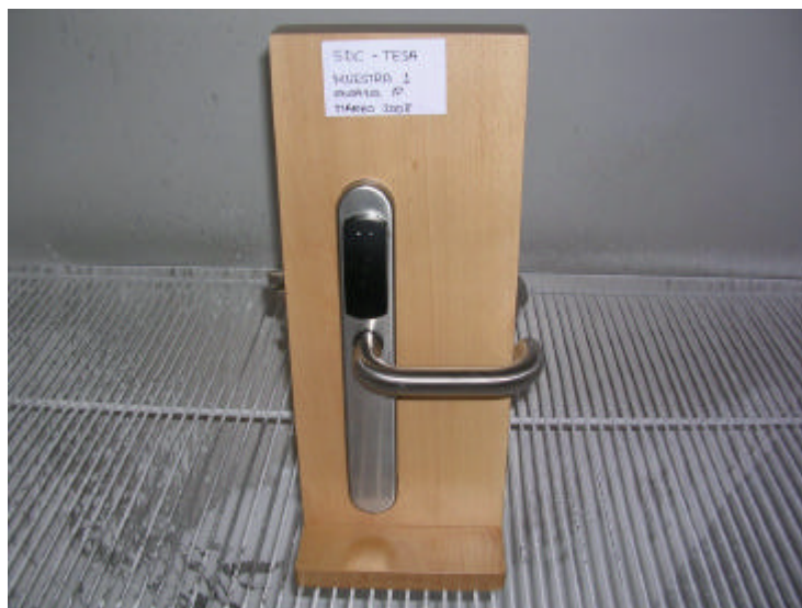
The equipment under test, for IP5X test.
