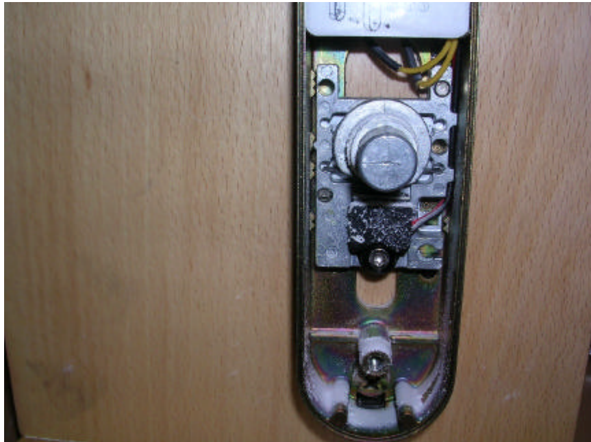
Inside equipment under test (at the bottom), ingress of talcum powder.
