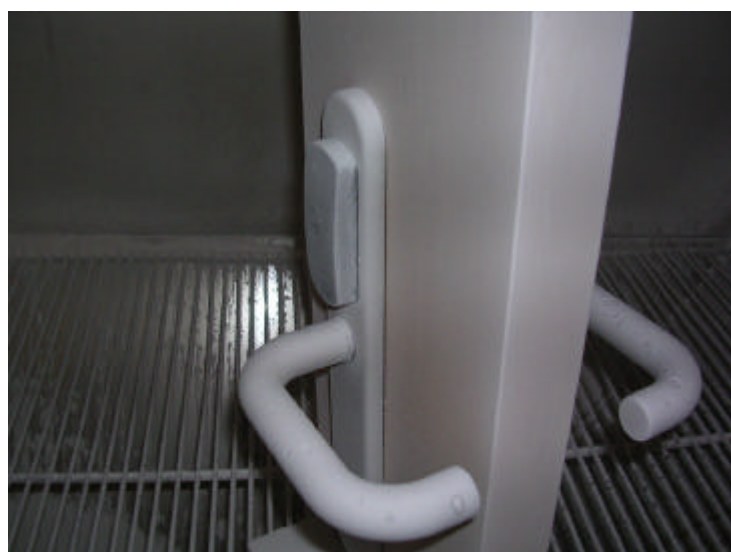
The equipment under test, after IP5X test.
