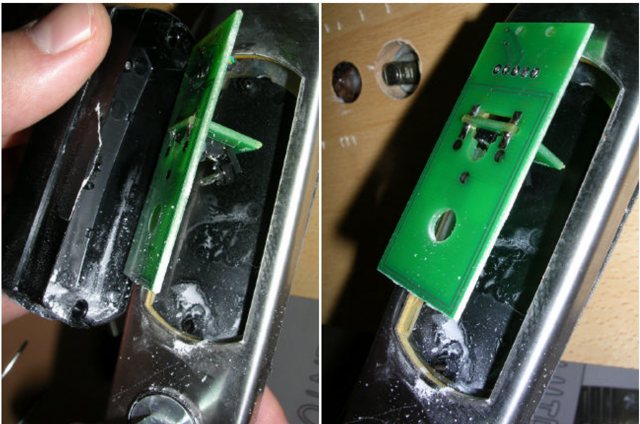
Inside the equipment under test (at the top), ingress of talcum powder.
