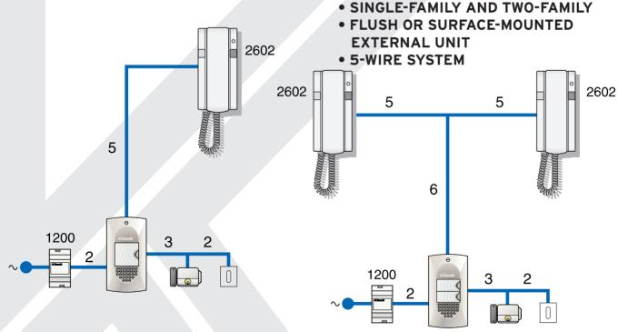
Style Kit 5 is the "ideal" door entry phone kit which uses 5 wires and is available in the single-family and two-family version. Style Kit 5 has an original and innovative design characterised by its unmistakeable and exclusive blue LEDs, by large name labels and by high sound quality. Simply by adding a telephone or an additional bell allows easy expansion and an elegant desk base ensures flexibility for all needs.
